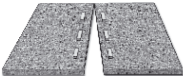
Blocks attached to the sheet
